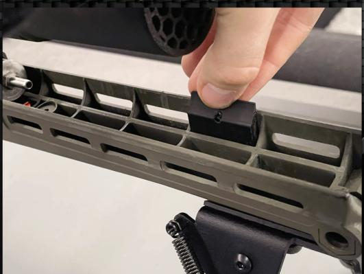
INSERT MOUNTING BLOCKS WITH THE ROUNDED EDGE FACING UP.
