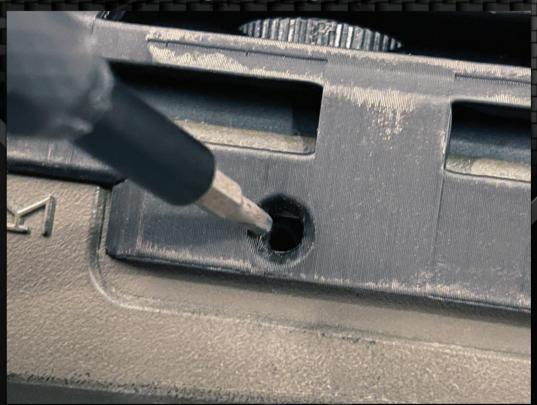
LINE UP THE MOUNTING BLOCKS WITH THE SCREW HOLES BY USING AN ALLEN KEY.
