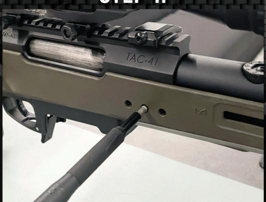
**UNDO THE 3 BARREL LOCKING** BOLTS.
